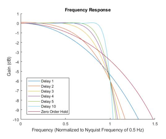
In the time domain, the interpolation does introduce some ringing in the step response of the antialiasing filter, which could affect some digital switching applications. However, the choice of **Number of samples of delay** parameter of 1 and **Output rise/fall time** parameter greater than zero is specifically designed to produce a smooth waveform transition with no ringing.
