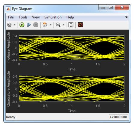
Open the configuration parameters dialog box. Change the **Symbols per trace** parameter to 4. Run the simulation and observe that four symbols are displayed.
